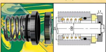
Vulcan manufacture and stock a range of single-spring stationary seals, with Silicon Carbide faced counter-ring rotaries, and inserted Carbon sprung-stationaries to replace the chrome-oxide coated rotaries of the O.E.M. seals.
