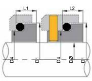
Common 'O'-Ring mounted stationaries to suit EURO-DIN housing sizes, designed to provide a wide range of compatability with Vulcan rotary seal types.
