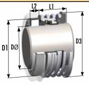
Robust, short working length, highly accommodating and reliable, rubber diaphragm balanced seal, which provides enhanced seal capability, performance and life. The A2 Type coil fits over the seal head, reducing the overall working length, making this seal suitable for short gland depth applications.
