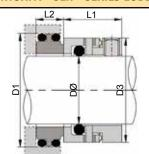
Vulcan manufacture and stock Type 1683 wave-spring 'O'-Ring mounted seals with bi-elastomeric Stationaries, to suit Inoxpa® SLR® series lobe-rotor pumps. As with the majority of lobe rotor designs, two seals are required for each pump.
