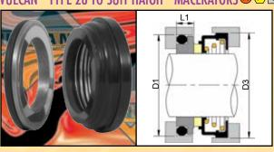
Vulcan manufacture and stock 1.1/4" rotaries, and 1.3/4" complete seals, to suit Haigh® macerators. Rotaries have Carbon faces with Nitrile elastomers, complete seals have a Ni-Resist cast iron stationary with a Nitrile 'O'-Ring.
