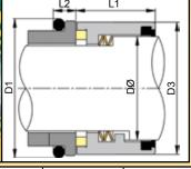
Vulcan manufacture and stock two sizes of hydraulically balanced, multi-spring hygienic seals to suit Variflow® TP-series pumps.
