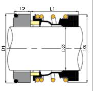
Vulcan manufacture and stock Type 192G elastomer bellows seals designed to replace the Grundfos® seal styles "A-" and B-" with a single, superior performing and easier to install seal design, in the majority of their centrifugal pump ranges.
