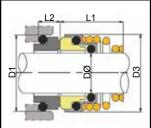
Vulcan manufacture and stock a 14mm Type 131 seal to suit the reduced length seal chamber of various circulating pumps, such as "CE-" and "CO-" ranges with newer "A" suffix motors. The Type 131 is the same dimensions to Vulcan Type 13, except for the reduced rotary working length.
