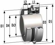
Stationary based, unitised elastomer bellows seals, utilised in small shaft diameter applications. Compact, unitised design, provides excellent flexibility in accommodating shaft mis-alignment and with quality seal face materials, to extend seal performance and life. The adequate shaft clearance enables one size to be used on a number of shaft sizes, whilst being stationary based increases the seals bidirectional rotational speed capabilities.
