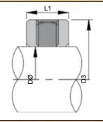
Stainless steel, grub-screwed, locking collars, utilised primarily for setting the working length to suit or fit the seal preferred.
