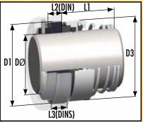
Conical spring, 'O'-Ring mounted, shaft directional dependent seal with inserted seal face and stationary to suit DIN housings. Type 8DIN has a 8DIN LONG stationary with anti-rotation provision, Type 8DINS has an 8 DIN SHORT stationary.
