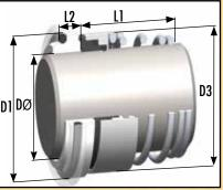
Resilient, conical spring, 'O'-Ring mounted, shaft directional dependent seal with a stationary to suit DIN housings.
