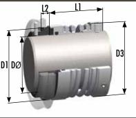
Robust, general purpose, unbalanced pusher-type 'O'-Ring mounted seal capable of many shaft-sealing duties. The Type 97 drives from the shaft, via the drive collar with grub screws, inserted in the spring coil tail.
