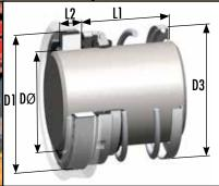
Metric shaft size, resilient, single spring, rubber diaphragm seal with a Type 20 boot mounted stationary as standard, to suit original common UK housing sizes. A widely utilised seal type, highly suited to general duties, capable of long service life.
