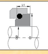
Common Vulcan 'O'-Ring mounted designs without anti-rotation provision, to suit common European housing sizes including DIN.
