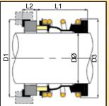
Vulcan manufacture and stock 32mm elastomer bellows seals with smooth-boot stationaries, to suit the extended seal chamber of S.P.P.® Eurostream® centrifugal pumps, commonly associated with large building service applications, such as heating and fire systems.
