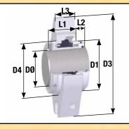
Modular design, Balanced, multiple spring, 'O'-Ring Mounted, two-bolt gland Cartridge Seal Assembly, with dual tangential flush as standard. Designed with minimal internal and external protrusion and with gland dimensions for near universal fitting.
