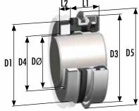
Stationary based, unitised elastomer bellows seals, utilised in small shaft diameter applications. Compact, unitised design, provides excellent flexibility in accommodating shaft mis-alignment and with quality seal face materials, to extend seal performance and life. The adequate shaft clearance enables one size to be used on a number of shaft sizes, whilst being stationary based increases the seals bi-directional rotational speed capabilities.
