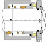
Vulcan manufacture and stock a range of single-spring stationary seals, with Stainless Steel counter-ring rotaries with outer turning-vane, and inserted Carbon sprung-stationaries.
