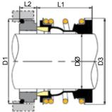
'O'-Ring mounted rubber bellows seals to DIN24960 / EN12756 dimensions, but with a balanced rotary face profile and special stationary profiles, to suit service in Andritz® "S-"series centrifugal pumps, commonly found in paper and cellulose processing.
