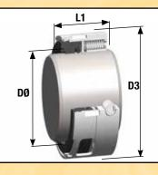
Narrow profile, metric shaft, multiple spring Seal with a highly efficient design. These Seals are frequently fitted with Type 24 DIN Long 'O'-Ring stationaries, see the opposite Page. Type 1659 incorporates a P.T.F.E. Wedge secondary Seal, Type 1659S is an 'O'-Ring Mounted design. Types 1659B and 1659BS are balanced designs for stepped-shafts.P.T.F.E. Back-Up Ring is recommended for higher pressure 'O'-Ring applications. The stock size code is always set by the shaft size under the Seal body.
