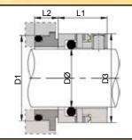
Vulcan manufacture and stock our Type 1688Y 'O'-Ring mounted wavespring seals, with the very distinctive seat outer profile.
