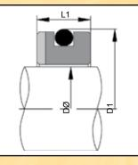
'O'-Ring mounted, monolithic 'H'- configuration stationaries, to suit common European housings (Type 21) or common American (Type 31) housing dimensions.
