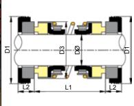
Rubber diaphragm double-ended seals with boot mounted stationaries, to suit the internal dimensions of Ebara® "Best-", "Right-" and "DW-" series, small submersible pumps. This common seal type is also utilised by other pump manufacturers for small portable submersible pumps.
