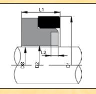
'L'-Shaped P.T.F.E. boot-mounted stationary, to suit common American housing sizes. Due to the low-friction nature of P.T.F.E., this stationary seat has necessarily been designed with an anti-rotation provision, and it is recommended to ensure this is utilised.
