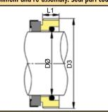
0444.1628.V.S.FACE Rotary Face with 'O'-Ring 0444.1628.V.S.STAT Stationary Seat 0444.1628.V.X.BOOT Stationary Cup Boot
