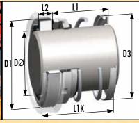
Compact, single spring, rubber diaphragm seal specifically designed to comply with DIN 24960 (EN 12756) L1K-length dimensional requirements, for the complete seal and seat assembly.
