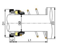
Vulcan manufacture and stock a variety of standard range seals to suit various Eureka® pumps (now part of Hamworthy®, formerly Thune-Eureka®). Type 277 is an elastomer diaphragm seal, with reverse taper seal to specifically suit the "CG-" series centrifugal pumps, widely used in marine applications.
