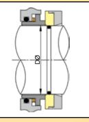
Vulcan manufacture complete single and double seals for the common FKL50 lobe rotor pump. The Vulcan design incorporates an inserted Silicon Carbide rotary, removing the O.E.M. chrome oxide rotary and providing a cleaner solution for food process. For further FKL series seals, please contact us.
