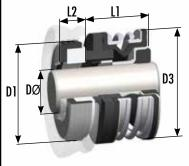
Sleeve mounted, rubber bellows seal with shaft drive ring. Similar to Type 60 but with dimensions to suit common American standards.
