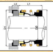
Rubber-bellows seals with boot mounted stationaries and Stainless Steel spacer-rings, to suit internal dimensions of Ebara® "EVM" and "EVMW" vertical multi- stage pumps.
