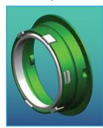
The drive area has been increased by over 250%, to greatly reduce the contact drive pressure and consequent wear. As a result, the drive ring does not cut nor groove into the seal head retainer
