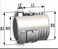
Robust, long working length, highly accommodating and reliable, rubber diaphragm balanced seal, which provides enhanced seal capability, performance and life. The Type A1 has a retainer backing plate, a narrow profile and a no spring base plate. Also now available for metric shafts.
