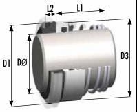
Conical spring, 'O'-Ring mounted, shaft directional dependent seal and stationary of similar design to the Type 8, but with a solid stainless steel head and 'O'-Ring mounted carbon stationary. Type 8B seal is supplied with a Type 8B seat as standard.
