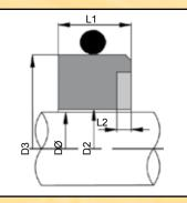
Monolithic stationary ring, with an 'O'-Ring installed in a radial groove outside of the stationary ring. This method of installation allows direct contact between the back of the stationary ring and the pump housing.
