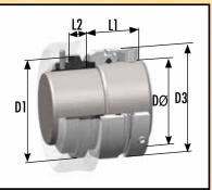
Stepped shaft, balanced sinusoidal wavespring, 'O'-Ring mounted seal, similar to Type 1677, most commonly utilised in higher-pressure pump applications. Vulcan Types 1677, 1677M and 1678 all have sinusoidal continuous wave-springs without joints or weld-spots, for maximum spring reliability.
