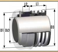
A robust rubber bellows seal, with a wide, larger than DIN, cross section, for optimum flexibility and durability. Type 19L is supplied as standard, with a Type 8 DIN LONG 'O'-Ring mounted stationary with an anti-rotation provision, to suit DIN housing dimensions.
