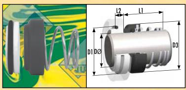
Conical spring, 'O'-Ring mounted, shaft directional dependent seal, with a monolithic rotary head. Supplied as standard with Type 8 STD stationary to suit European non-din housing sizes.
