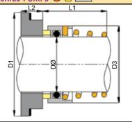
'O'-Ring mounted conical spring 22mm seals with distinctive gasket mounted seat rings, to suit "SOB" and "SOH" series pumps, commonly found in ship's engine rooms.
