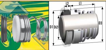
'O'-Ring mounted, conical spring, shaft directional dependent seal, with pressed stainless steel head retainer and 'O'-Ring mounted seal and stationary faces.
