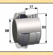
Narrow profile, multiple spring, 'O'-Ring Mounted, set screw driven, non-clogging, Balanced Mechanical Seal. The Balanced design, protected springs sealed out of the fluid and dynamic 'O'-Ring enable use in demanding applications. A P.T.F.E. Back-up Ring is recommended to be specified for higher pressure applications.
