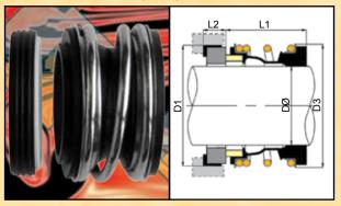
Vulcan manufacture and stock a range of elastomer bellows seals to suit the specific dimensions of K.S.B.® "AMA-", "KRT-" and "SEWA-" series waste-water pumps with "SU-" prefix seals installed. 25mm size is commonly used in the 'oil bath' position, with 22mm Type 19B found on page 45 in the 'outer' position, 33mm sizes are used in pairs in the same pump series. 28mm is commonly used in "Vitachrom" numps in tandem with Type 127B
