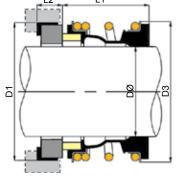
Vulcan manufacture and stock 22mm elastomer bellows seals with special profile boot mounted Stationaries to suit Grundfos® "LM", "LP, LPD and LPE" series pumps. Widely utilised in building service applications.
