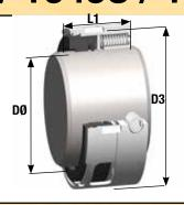
Narrow profile, multiple spring Seal, designed for the common American ANSI B73-1974 Centrifugal Pump standard. Frequently fitted with Type 23 P.T.F.E. Boot Stationary. Type 1645 utilizes a P.T.F.E. Wedge secondary Seal, Type 1645S is 'O'-Ring Mounted design, Types 1645B and 1645BS are balanced designs for stepped-shafts.
