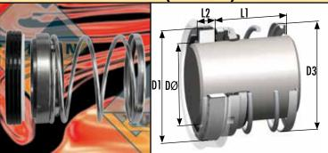
Single spring, rubber diaphragm seal, similar to Type 11/22, but with reduced 0.D. (D3) to give full ANSI seal chamber compatibility. Type N11 / N22; with a resilient elastomer mounted face, is the preferred design supplied up to its design limit of 2.000" / 50 mm. Type U11 / U22 has a retainer lug driven face, as per our Type 24 design and is the preferred design, that is supplied in all sizes above 2.000" / 50 mm. Also available as Types N11J / N22J or U11J / N11Jwith an '0'-Ring mounted seat.
