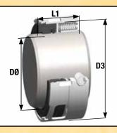
Multiple Spring Seal with a highly effective design, commonly used in chemical and petrochemical duties. Frequently fitted along with the Type 25 clamped Stationary. Type 1609 incorporates a P.T.F.E. Wedge secondary Seal, Type 1609S is an 'O'-Ring Mounted design. P.T.F.E. Back-Up Ring is recommended to be specified for higher pressure 'O'-Ring applications. Types 1609B and 1609BS are designed for stepped shafts.
