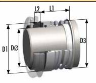
Robust, general purpose, unbalanced pusher-type, 'O'-Ring mounted seal, capable of many shaft-sealing duties. The Type 96 drives from the shaft via a split ring, inserted in the coil tail.
