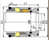
Vulcan manufacture and stock multi- spring seals to replace the original O.E.M. wave-spring seals, utilised for hygienic applications in Grundfos® Hilge® centrifugal pumps.
