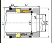
Vulcan manufacture and stock two sizes of hydraulically balanced, multi- spring hygienic seals to suit Variflow® KN-series pumps, directly replacing the original design.
