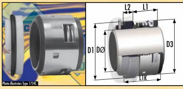
High performance, rubber bellows seal inside a stainless steel casing. Type 1724 features a retained, positively driven, face with a non-clogging spring and selfalignment capability, and is fully compliant to DIN24960 (EN12756) dimensions.
