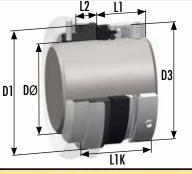
Sinusoidal wave-spring, '0'-Ring mounted seal commonly utilised in the European chemical process industries. Manufactured to suit DIN24960 (EN12756) dimensions.
