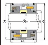
The Vulcan Type 1640 is a direct replacement for the older-generation "EBS" O.E.M. seals. Newer pumps have a slightly modified seal installed, which is directly replaced by the Vulcan Type 1642. Please check the outer dimensions of the seat housing for correct identification, utilising the table below, D3 dimension.
