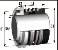
A robust rubber bellows seal, with a wide, larger than DIN, cross section, for optimum flexibility and durability. Type 19S series seals are supplied as standard with Type 8 DIN SHORT '0'-Ring mounted stationaries to suit DIN 24960 (EN12756) housing dimensions.
