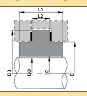
The Type 25 stationary is an industry standard design with a "T"-shaped profile. Supplied complete with two P.T.F.E. flat gaskets, for clamping as illustrated. The Type 25 is designed for medias that are aggressive towards elastomers, and is widely utilised with Type 1609/1645/1659 series multi-spring rotaries. For shaft sizes up-to 1.000"/25mm; please add 1.60mm to dimension L2 for the gaskets width, similarly add 3.20mm for shaft sizes 1.125"/28.00mm and above.
