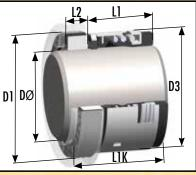
High performance, heavy duty, full convolution rubber bellows seal inside a stainless steel casing. Type 1724 features a retained, positively driven, face, with a non-clogging spring and self-alignment capability, and is fully compliant to DIN24960 (EN12756) dimensions.
