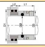
Vulcan manufacture and stock our Type 1688Z 'O'-Ring mounted wavespring seals with bi-elastomeric stationaries, to suit "Top Lobe®" series lobe-rotor pumps.
