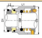
Vulcan manufacture and stock a 22/26mm step-balanced, 'O'-Ring mounted, robust single spring seal with positive drive from three drive studs on the coil base, to suit larger models of "SV- and e-SV-" series pumps.
