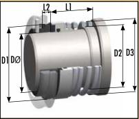
Robust, general purpose, unbalanced pusher-type, 'O'-Ring mounted seal, capable of many shaft-sealing duties. The Type 95 drives directly from the shaft, via a raised area of the shaft.
