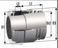
Conical spring, 'O'-Ring mounted, steppedshaft, balanced, shaft directional dependent seal. Supplied as standard with Type 8 DIN LONG stationary with anti-rotation provision. The standard seat size for each seal size is shown in the table below.
