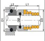
Vulcan manufacture and stock 38mm 'O'-Ring mounted conical spring seals, in clockwise and anti-clockwise rotation, to suit the housing dimensions of common Sterling Sihi® pumps.
