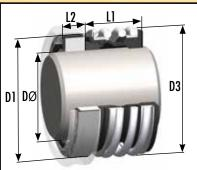
A robust rubber bellows seal, with a wide, larger than DIN, cross section, for optimum flexibility and durability. Type 19B series seals are supplied as standard with Type 19B boot mounted stationaries to suit DIN 24960 (EN12756) housing dimensions.
