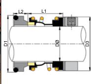
Vulcan manufacture and stock 16mm elastomer bellows seals with spacer and clamp ring to suit the Grundfos® "CP" series pumps. Widely utilised in building service applications.
